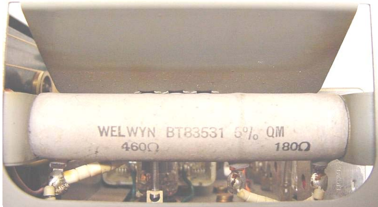
The mains dropper (ballast), R20, switched into the power supply circuit on 210v and 240v supply positions
